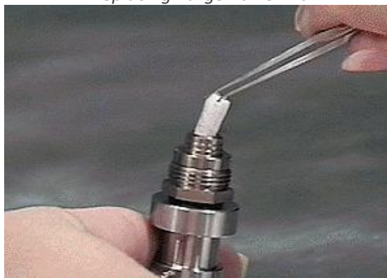
Figure 6-10 Replacing Purge Valve Frit
